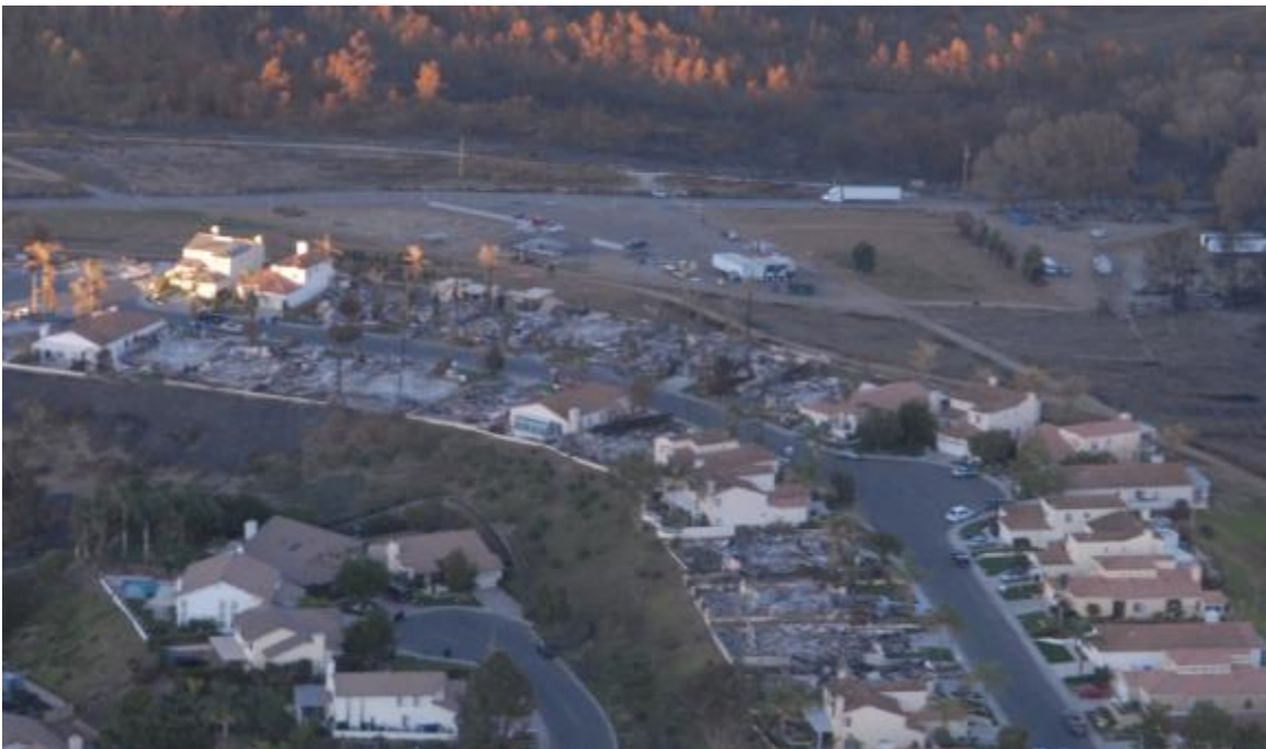
2007 Witch & Guejito Fire Locations showing rural open space where fires began as well as clustered homes which burned due to house to house spread
